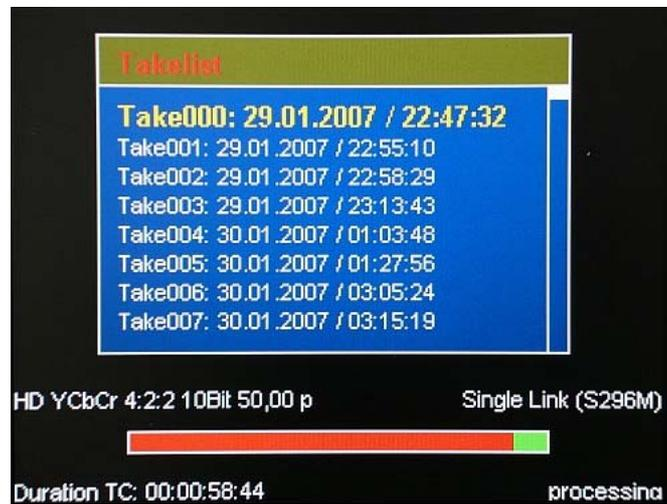
In the take list all takes are listed with their recording time. Using the buttons UP / DOWN a take can be selected. The recorded format for the selected take will be displayed in the area above the capacity bar. Pressing „OK“ chooses the selected take as the currently selected take.
