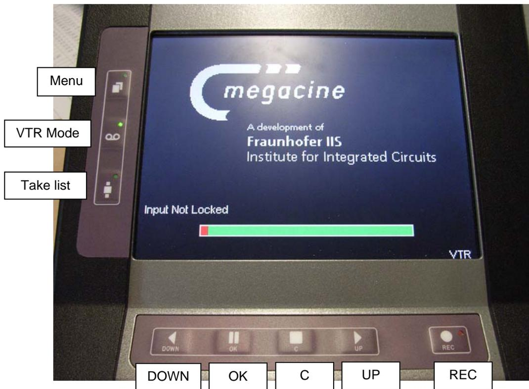
There are 9 controls (8 push-buttons + 1 switch) on the unit:
