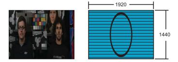
To output this oversized image it is split into two HD 4:2:2 streams. Each HD stream contains a 1920 x 720 letterbox image in 2.66:1 aspect ratio (180 blank lines on top and bottom). Stream A contains all odd lines (line count starts from 1), stream B all even lines of the original image.
